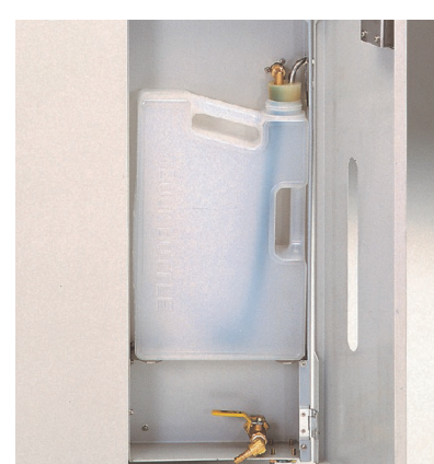
Drain bottle and drain valve
